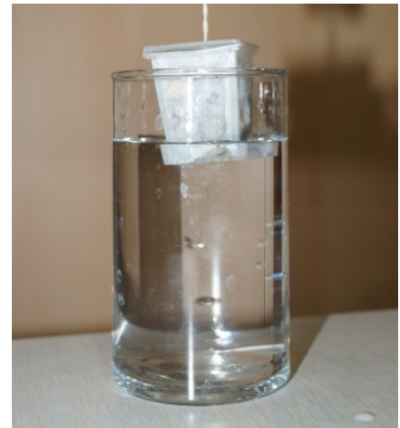
This water purifier uses silver-imbedded pebbles to produce potable water.
