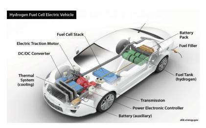
Fuel cell electric vehicles produce no tailpipe emissions, only water vapor and warm air. They can travel 300 to 400 miles on a tank of hydrogen and can refuel in three to five minutes.
